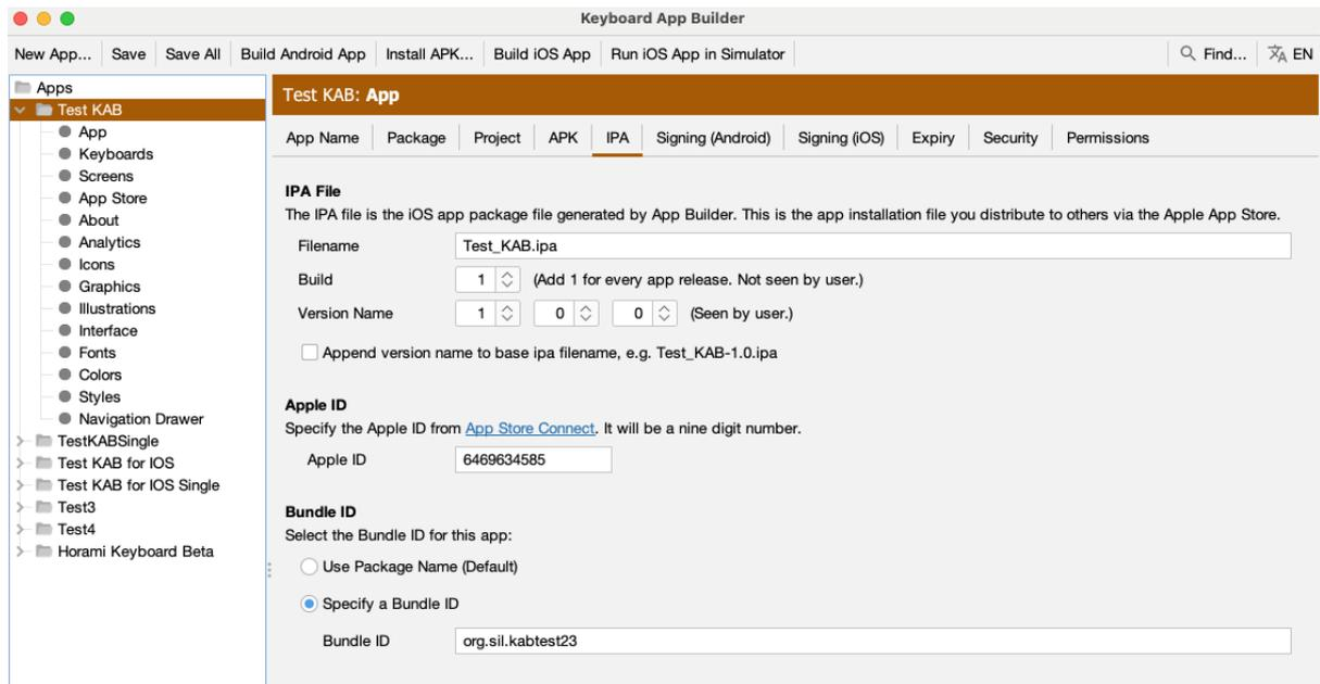
The **Filename** field on the screen for the **IPA File** section specifies the base name of the ipa file to be generated. If the checkbox at the bottom of the screen for *Append version name to ipa filename* is checked, then the version indicated by the *Version Name* fields is added to the base filename.
