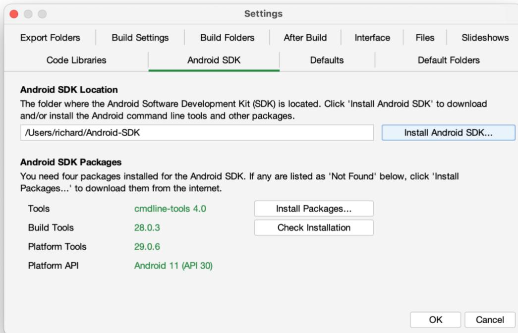
If any of the Build Tools, Platform Tools or Platform API is listed as “Not Found” (displayed in red), click the **Install Packages** button to install them.
