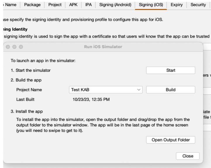
Pressing the **Start** button will start an instance of the iPhone simulator installed with XCode.
