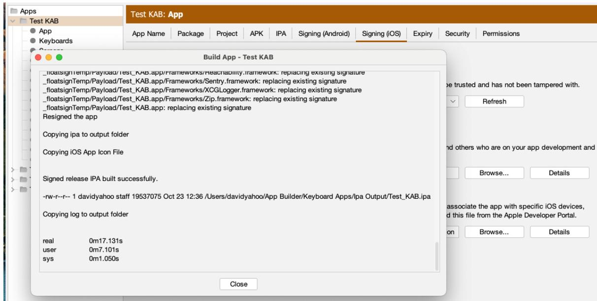
Examine the log window once the script has been completed. The message “Signed release IPA built successfully.” should appear in the window if the app has been build successfully.
